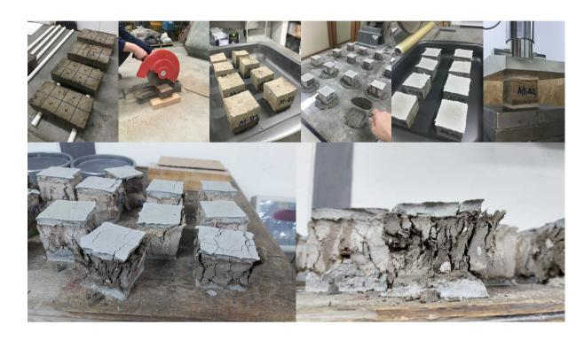
1.5MPa. On the other hand, according to the UNE 41410:2008 standard, we can affirm that the results obtained for samples B2 and B2 correspond to the BTC5 classification (resistance greater than 5MPa) while sample B1 corresponds to BTC1 (resistance greater than 1.3MPa).
