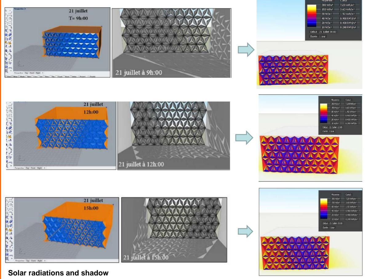
Before the integration of the dynamic facade, we observed a high direct solar radiation on the south facade. The radiation values range between 80 W/m<sup>2</sup> and 150 W/m<sup>2</sup>. These excessive radiation values have decreased remarkably with the dynamic protection of about 20 to 40 W/m<sup>2</sup>. This corresponds to a decrease of 27% of direct solar radiation,
